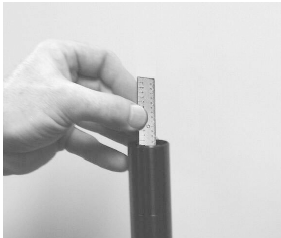
Figure K-8. Measuring the distance from the top of the flow adapter or sample tube to the top of the flow splitter.
