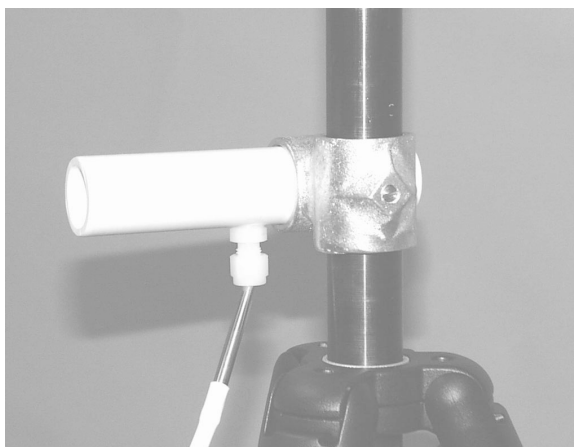
Figure 2-64. Installing the ambient temperature sensor into the ambient temperature sensor mount.
