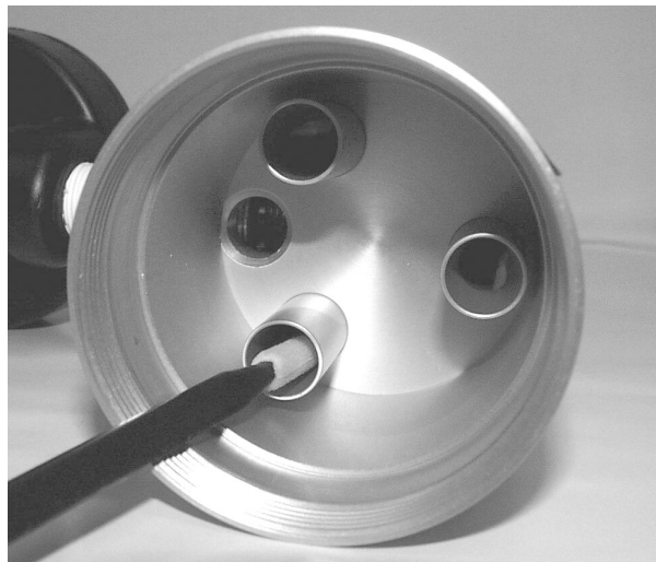
Figure G-10. Cleaning the vent tubes of the lower inlet assembly.
