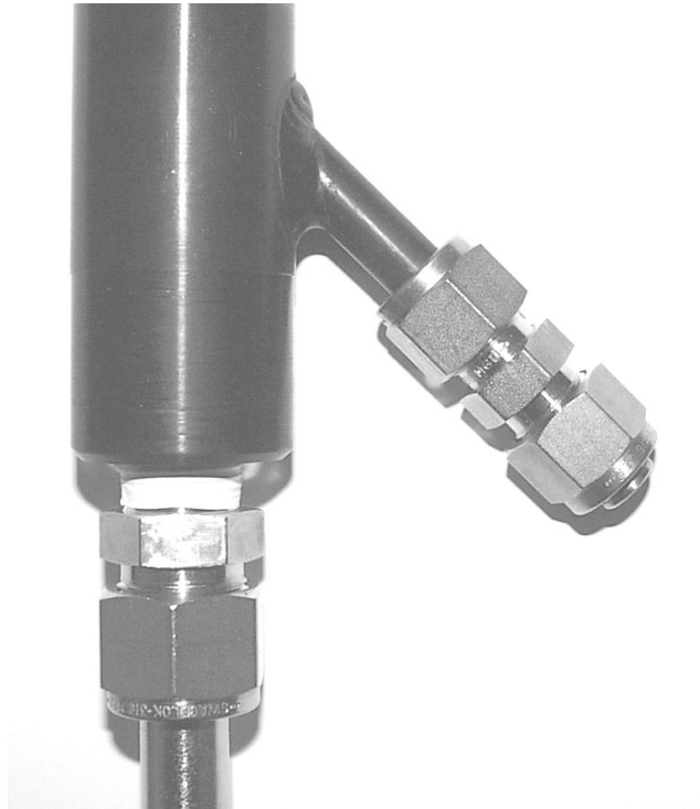
Figure 5-16. Bypass flow extension with 3/8-inch Swagelok cap.
