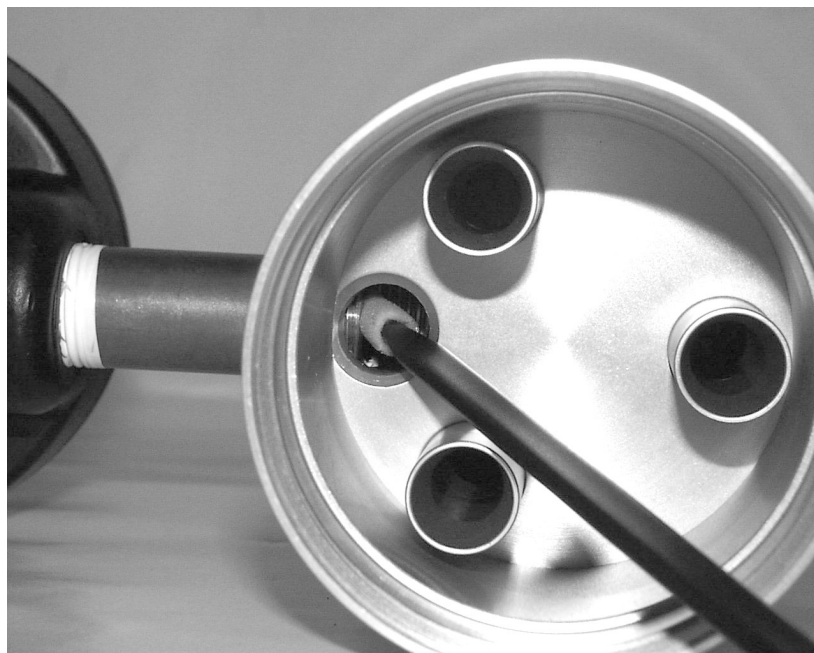
Figure G-12. Cleaning the weep hole in the collector plate.
