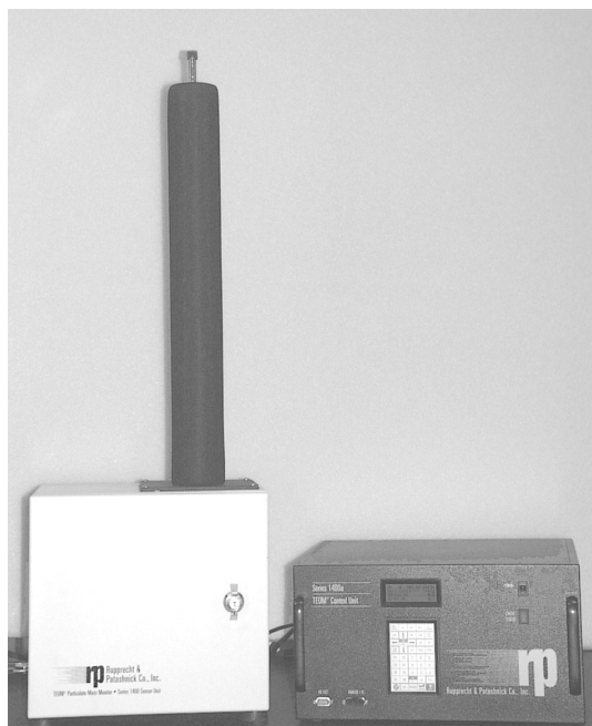
Figure 1-1. TEOM Series 1400a Ambient Particulate Monitor: sensor unit (left) and control unit (right).
