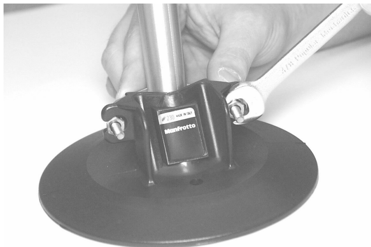
Figure 2-49. Tightening the metal bracket onto the tripod foot.
