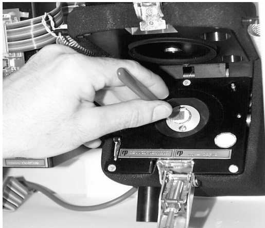
Figure 3-22. Removing a TEOM filter.
