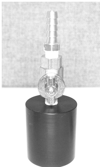
Figure 12-19. Flow audit adapter with valve open.
