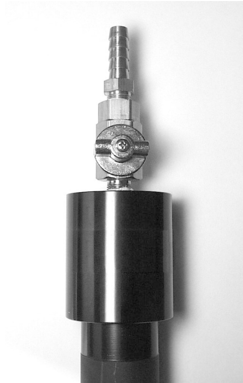
Figure 3-34. Flow audit adapter installed on flow splitter with valve closed.
