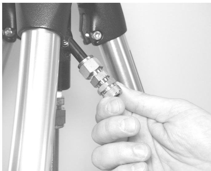
Figure 2-56. Removing the fastening nut from the bypass extension.
