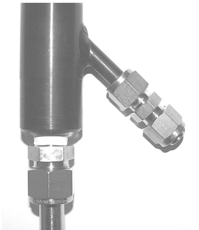
Figure 12-23. Bypass flow extension with 3/8-inch Swagelok cap.
