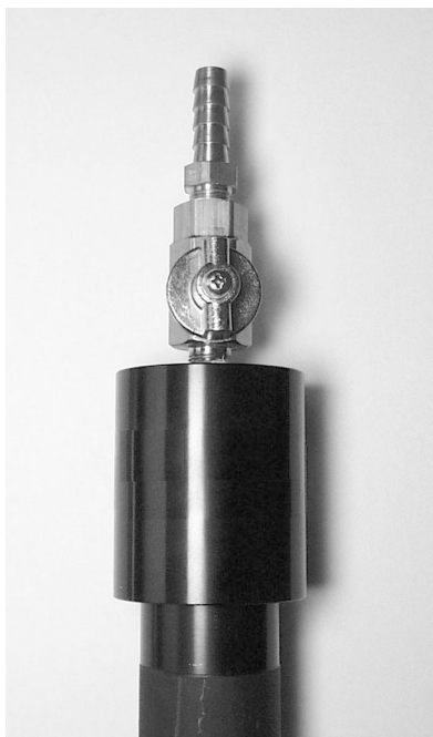
Figure 12-20. Flow audit adapter installed on flow splitter with valve open.
