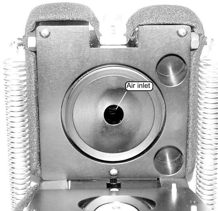
Figure 12-10. Air inlet inside the mass transducer.
