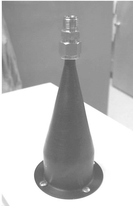
Figure 14-7. Sample distributor cone installed on top of the ACCU System enclosure.
