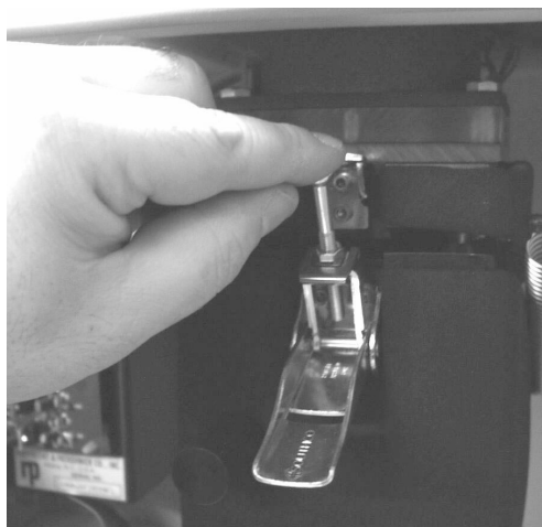
Figure 12-7. Releasing the holding rod on the mass transducer.
