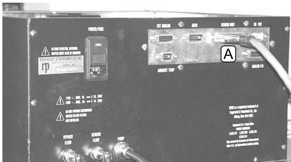
Figure 2-21. Back of control unit with the electric- and air-connecting cable attached to the “SENSOR UNIT” connection (A).
