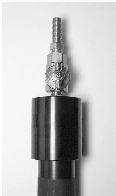
Figure 3-33. Flow audit adapter installed on flow splitter with valve open.
