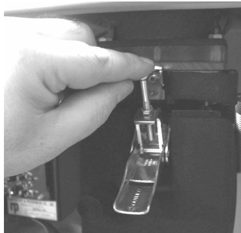
Figure 3-7. Releasing the holding rod on the mass transducer.
