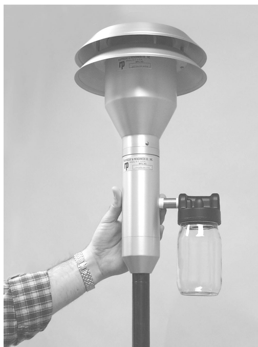
Figure 12-18. Removing the PM-10 inlet.
