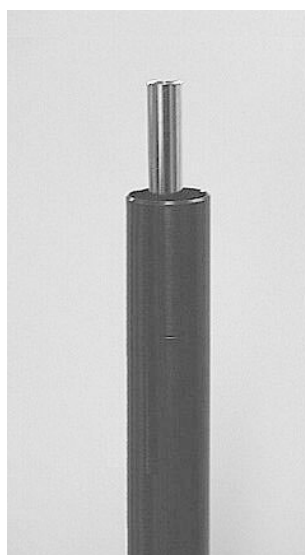
Figure 2-40. Sample tube positioned above the top of the flow splitter.
