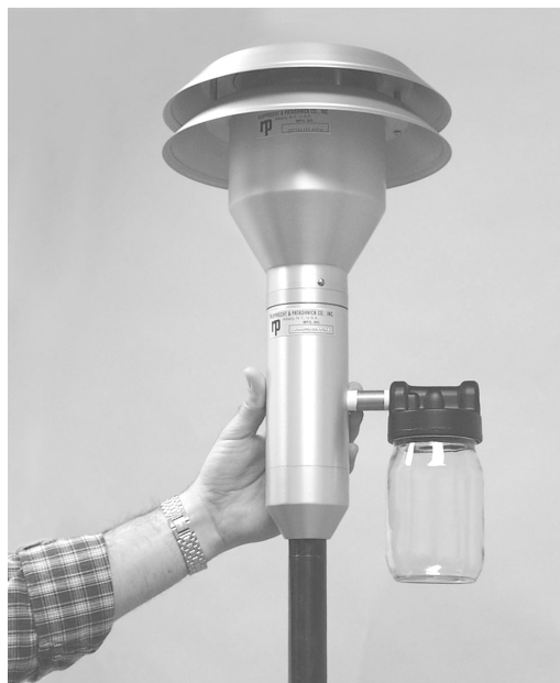
Figure 5-11. Removing the PM-10 inlet.
