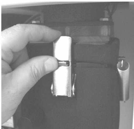
Figure 3-5. Lifting the shipping latch on the silver handle.
