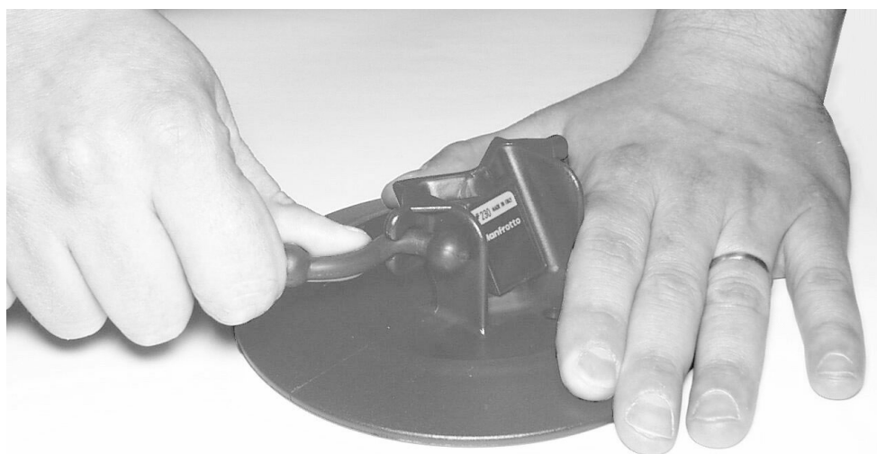
Figure 2-45. Removing the rubber leg holder.
