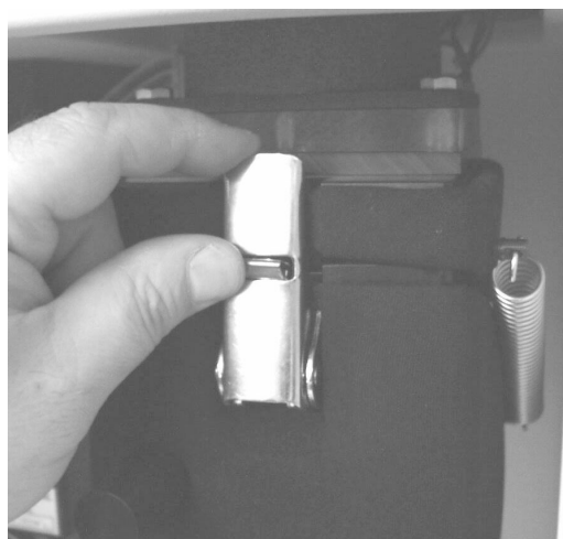
Figure 12-5. Lifting the shipping latch on the silver handle.
