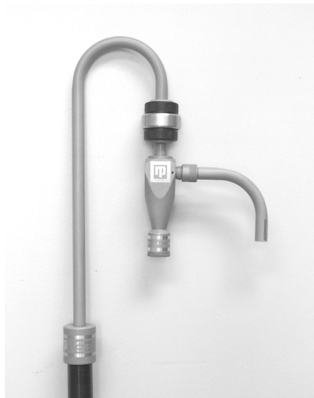
Figure 2-76 (right). U.S. TSP inlet (16.7 l/min) installed onto a flow splitter.
