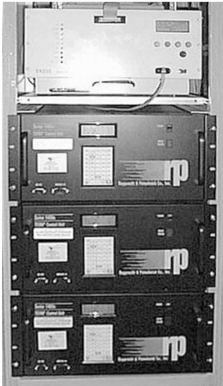
Figure 2-31. Three TEOM control units installed in a rack.
