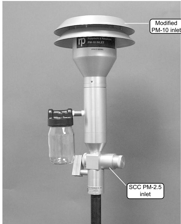
Figure G-17. Modified PM-10 inlet installed onto a sharp cut cyclone (SCC) PM-2.5 inlet.
