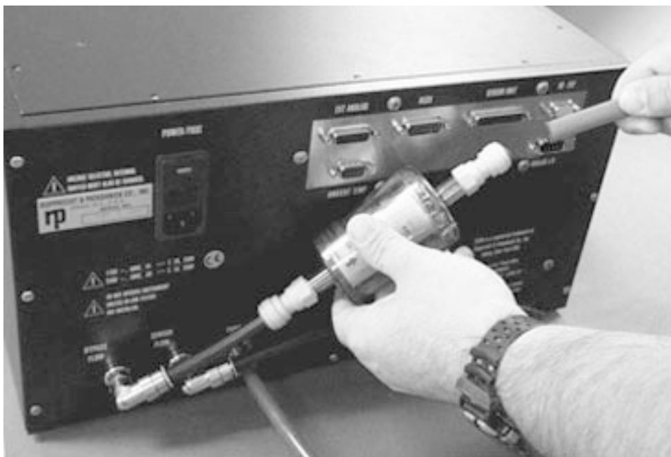
Figure 12-1. Replacing the large in-line filters.
