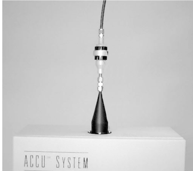
Figure G-24. In-line PM-2.5 ACCU inlet installed on the sample distributor cone.
