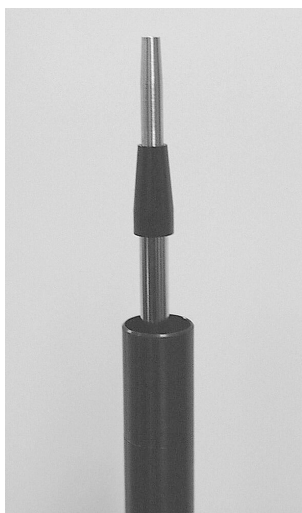
Figure 2-42. 1 l/min flow adapter installed on the sample tube.
