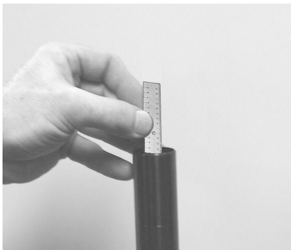
Figure 2-43. Measuring the distance from the top of the flow adapter or sample tube to the top of the flow splitter.
