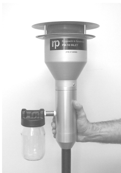
Figure 2-79. Removing the PM-10 inlet from the flow splitter.
