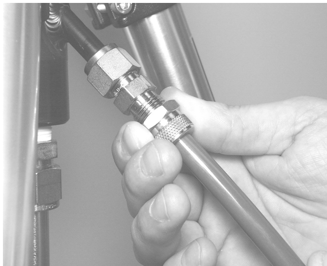
Figure 12-22. Disconnecting the bypass flow line from the bypass extension.
