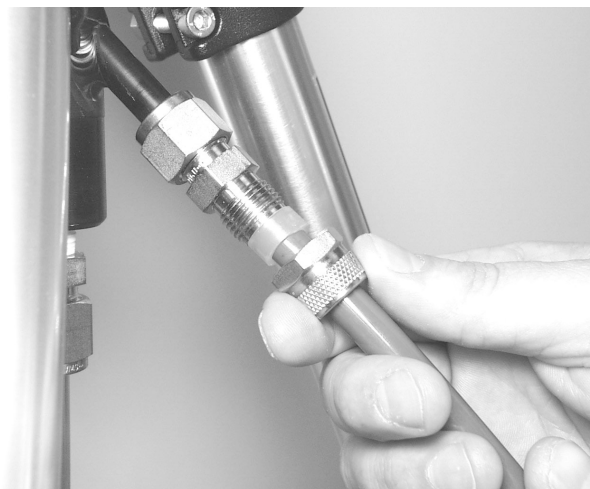
Figure 2-59. Installing the green bypass tubing onto the bypass extension.
