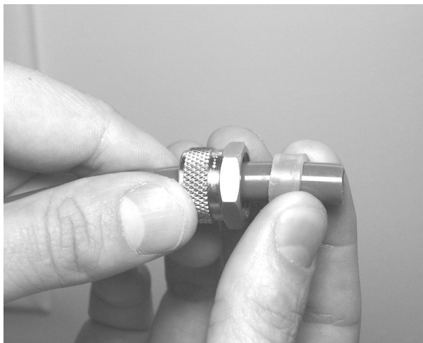
Figure 2-58. Installing the bypass extension and rubber ring onto the green bypass tubing.
