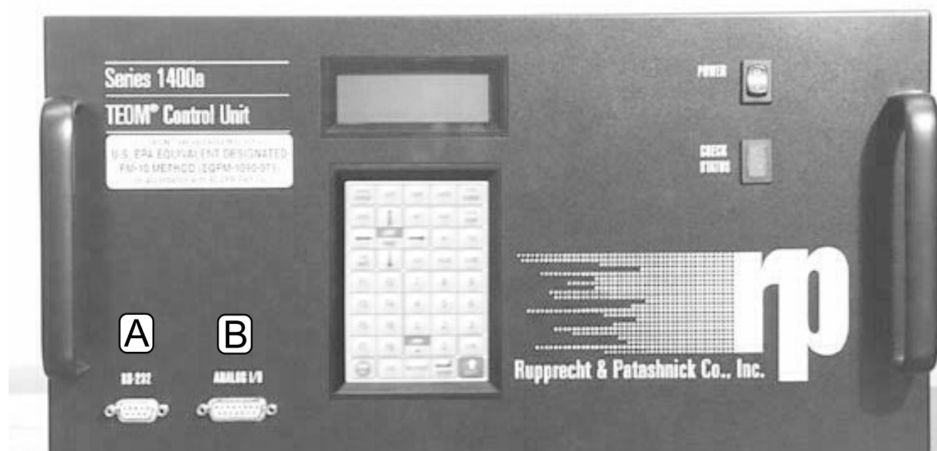
Figure 9-2. Front view of the control unit with the 9-pin RS232 serial connector (A) and the 15-pin analog connector (B) highlighted.
