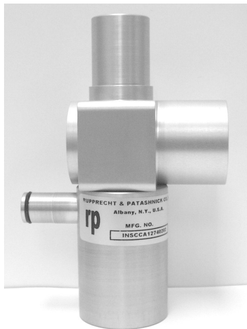
Figure G-21. SCC chamber with emptying cup, transfer tube and top cap removed.
