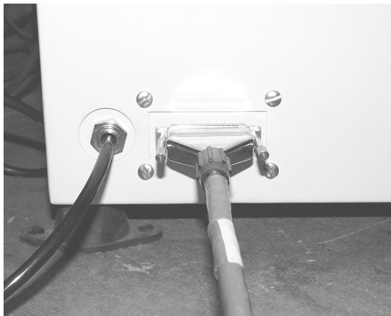
Figure 2-32. Electric- and air-connecting cable installed on the sensor unit.
