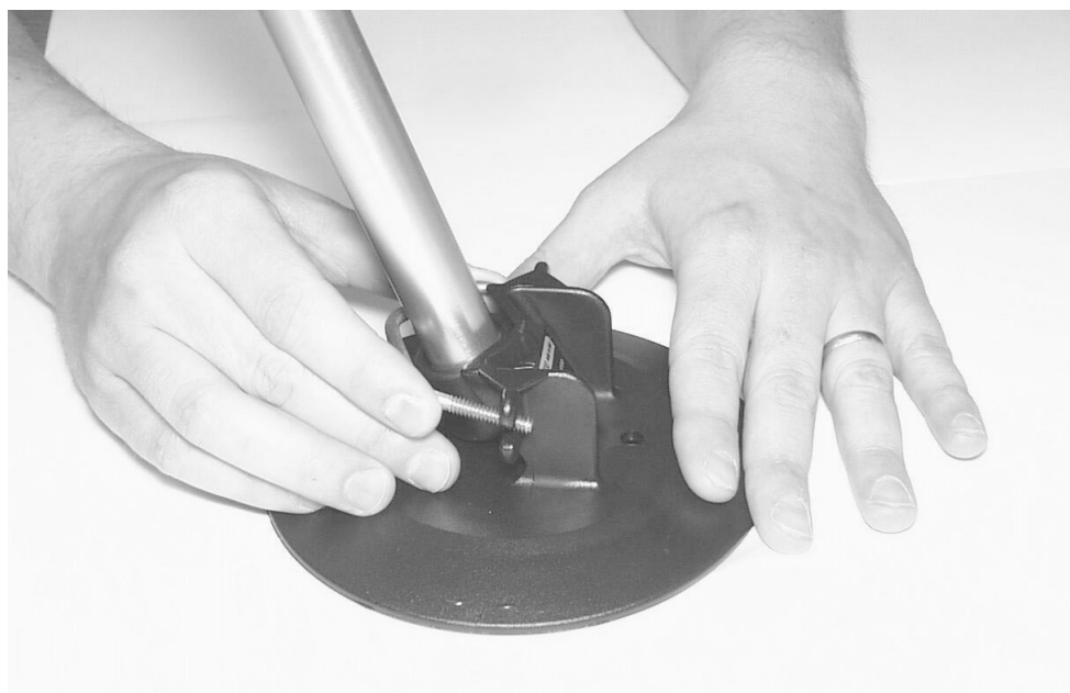
Figure 2-46. Placing the metal bracket on the tripod foot.
